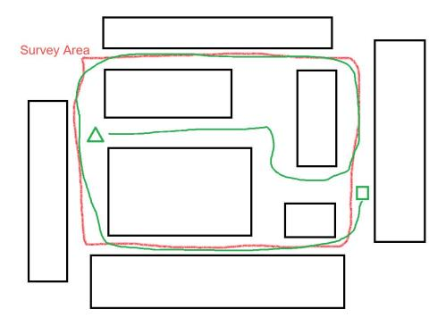
This route is suitable for small areas. However, in a large area, cumulative errors of the LiDAR IMU may cause point cloud stratification and deformation to occur.
