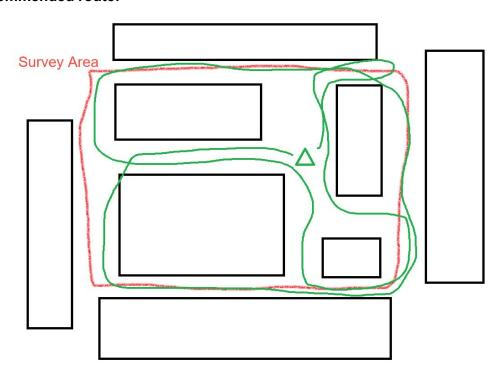
Try to start initialization at a location where the general structure of the whole survey area can be captured easily (such as the green triangle on the figure above). After initialization, scan the survey area one section at a time with small loops (as
